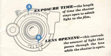
In general, an exposure time of 1/100 second or 1/50 second should be used for pictures made outdoors in sunlight. A short exposure time helps prevent blurred pictures which may result from a slight movement of the subject or the camera when you snap the picture.
