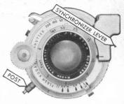
Class F Lamp is synchronized without use of the lever.
