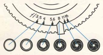
The illustration above shows how the size of the lens opening—the opening through which light passes to the film—is changed as the lens opening lever is moved across the scale.
