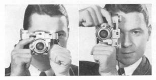
**Hold the camera steady.** If it is moved during the exposure, the picture will not be sharp. It's a good idea to hold your breath for an instant as you press the exposure lever.
